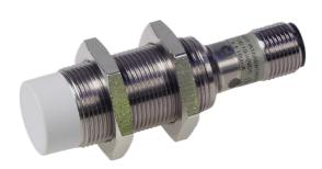
IA Series Inductive Proximity Sensors, non-flush type, nickel-plated brass M18 short housing, 10 to 40 V DC power supply, NC output, 14mm sensing range, IP67 rating, M12 plug, with 5m cable included
